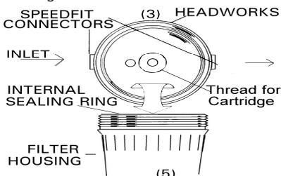
To seal the cartridges into the headwork's within the plastic housing, the upper spigot/thread of the cartridge threads into the headworks using the candle-sealing washer (5). THIS SEAL IS ESSENTIAL TO THE CORRECT WORKING OF THE FILTER. Develop the habit of checking that it is in place before you screw on the cartridge when you clean or change the cartridge.
