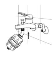
1) Screw the extension elbow into the shower filter
